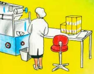
This machine finishes the job by putting the blister packs of tablets into cartons.
